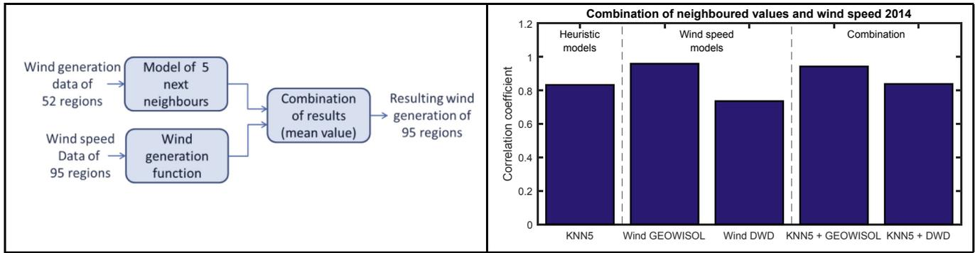
Fig. 8. The strategy of combining neighbored wind generation data and wind speed data (left) and calculated correlation values of single and combined methods (right).
